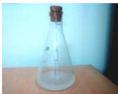
Figure 5: Reaction setup of CO 2 evolution assay showing the hanging tube containing 0.1(N) NaOH
